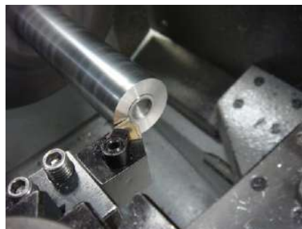
Gambar Proses bubut muka (sumber: restlessmass.com)
