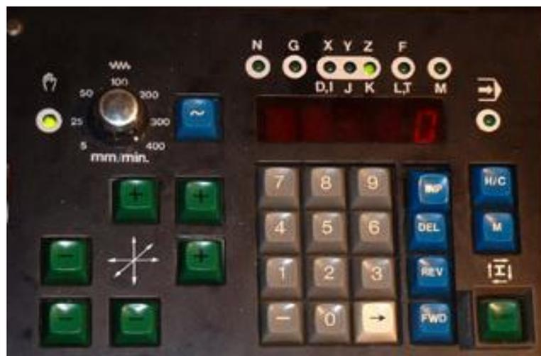
Gambar 1. Keyboard Mesin CNC TU-3A
