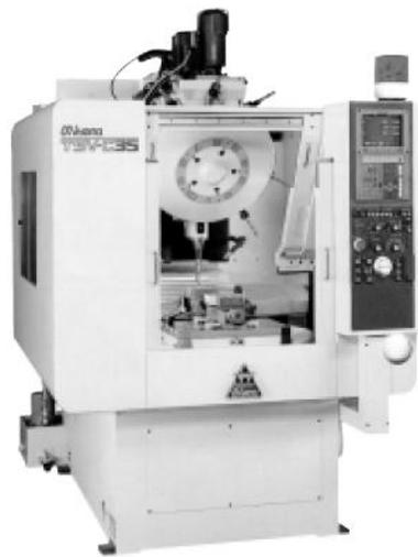
Gambar 4.2. Mesin Gurdi Radial (*Radial drilling machine*) dan Mesin Gurdi dan tap CNC (*Drilling and Tapping CNC Machine*)
