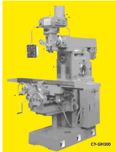
Gambar 7.2. Mesin Frais turret vertical horizontal.
