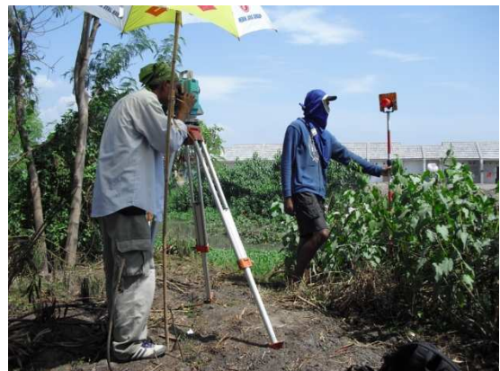
Figure 1. Surveying using Electronic Total Station (courtesy of CV Putra Mandiri)
