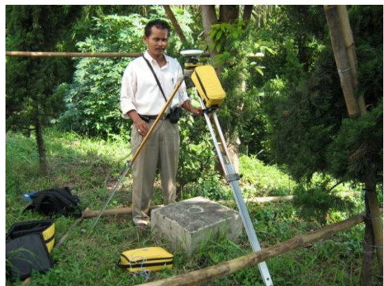
Figure 2. Surveying using GPS (courtesy of CV Putra Mandiri)
