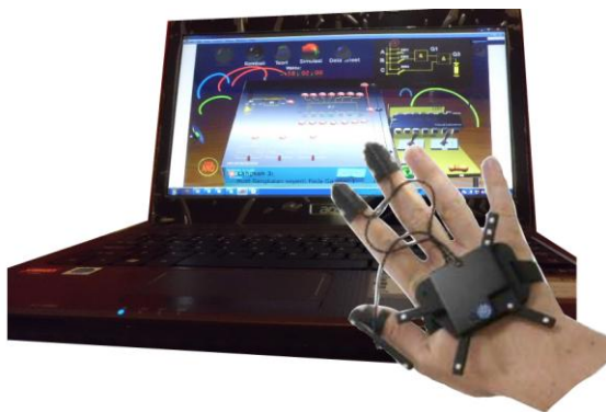
Figure 10. Virtual Laboratory Through Hand Motion Detectors (Hardware)
