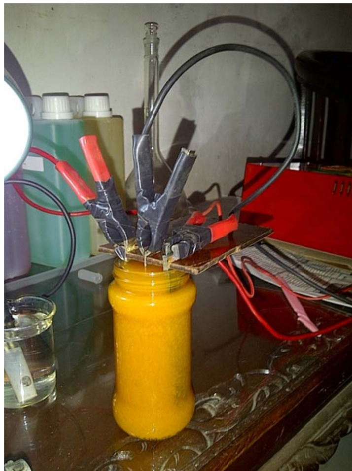
Gambar 2. Proses coating Fe-Co-Ni pada substrat stainless steel
