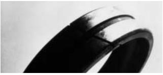
Figure 26. Pits Caused By Electrical Current
