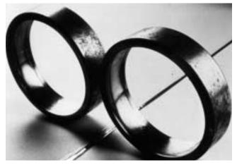
Figure 22. Smearing on a Bearing Race
