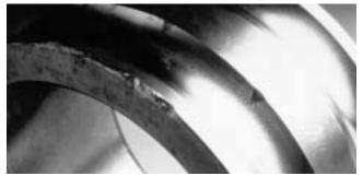
of serious fretting corrosion. Microscopic movement between the shaft and the bore causes the rust colored patches to develop. Small amounts of fretting are common with setscrew mounted bearings and are not detrimental to bearing life. Advanced cases, caused by loose mounting, can lead to cracks.
