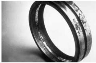
Figure 15. Bearing Roller with Rusty Ends Due to Moisture in the Lubricant
