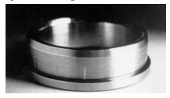
Figure 20. Spalls Resulting from True Brinneling
