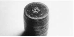
Figure 16. Puddle Corrosion
