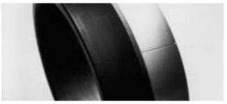
Figure 25. Cracked Outer Race
