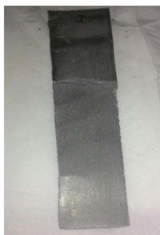
Figure 3b. Shape of aluminum after electrocoagulation
