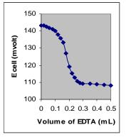
Figure 5: Potentiometry titration 25 mL  $10^{-5}$  M La<sup>3+</sup> with 5.10<sup>-3</sup> M EDTA by ESI-lanthanum
