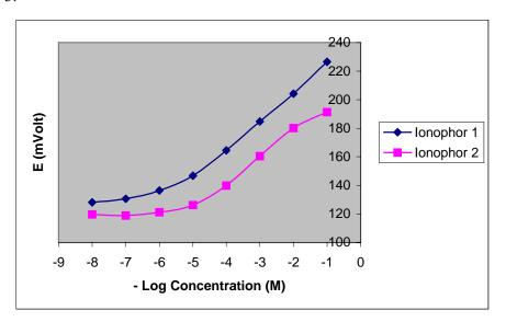
(ionophore 2). The capability of the electrode can see with response potential in figure 3.
