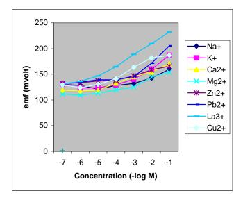
Figure 4: Potential response of La-ISE to ion  $\text{La}^{3+}$  and others From the data in figure 4, the value  $K_{A,B}^{Pot}$  is calculated with MPM system. The result for all ion interference can see in table 2.
