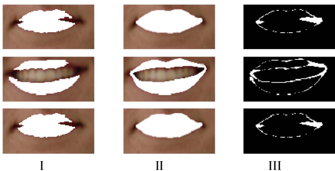
Fig.4. Example of lip segmentation and tracking using k-means where the inputs are Cb and Cr components in YCbCr color space, (I) automatic segmentation, (II) manual segmentation, (III) False Positive and False Negative
