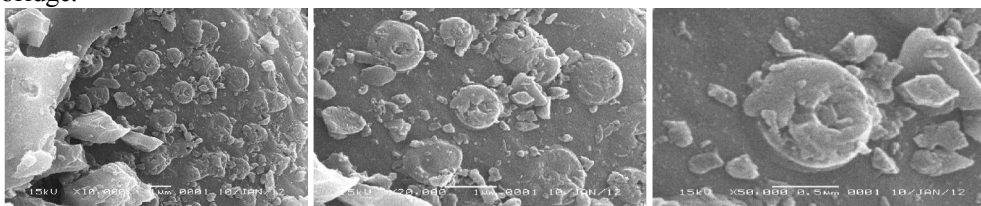
Figure 3. SEM micrographs of coconut shell carbon (5% wt. PVA) sintered 1500 °C
