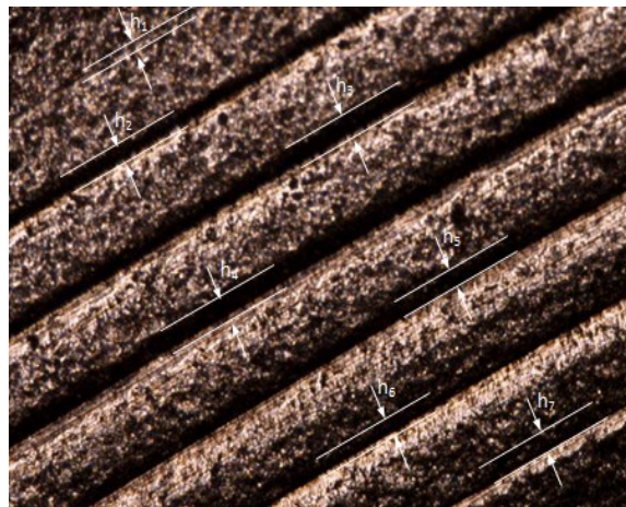
(c) surface roughness of gasket after contact with flange having surface roughness 2.5μm
