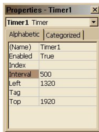
Figure-10 Change Interval value in Timer1 to select speed of program response.
