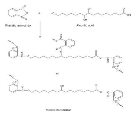
Figure 2: Chemical Structure of Modificated Matrix by Using Anhydride Phthalic
