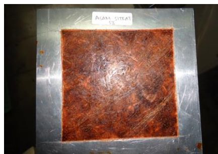
Figure 6. Preparation of biocomposites in mold
