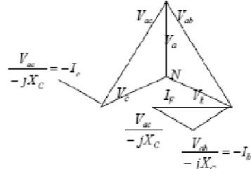
$$I_F = \frac{V_{ab}}{-jX_C} + \frac{V_{ac}}{-jX_C} = \frac{3V_{aN}}{-jX_C} \rightarrow 3x \text{ arus charging normal}$$
