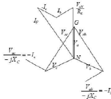
$$|I_b| = \sqrt{3} \left| \frac{V_b}{X_c} \right| \rightarrow \sqrt{3}x \text{ arus charging normal}$$
