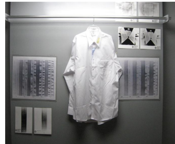
Test DP Rating
