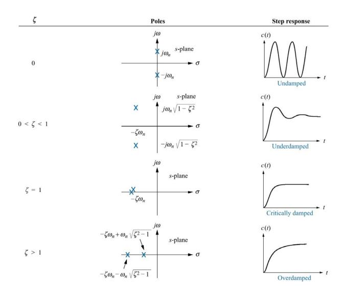
**Example:** Given the transfer function  $G(s) = \frac{\omega_n^2}{s^2 + 2\zeta\omega_n s + \omega_n^2}, \text{ find } \zeta \text{ and } \omega_n.$
