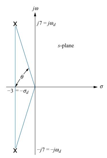
For the system shown, find J and D to yield 20% overshoot and a settling time of 2 seconds for a step input of torque T(t).
