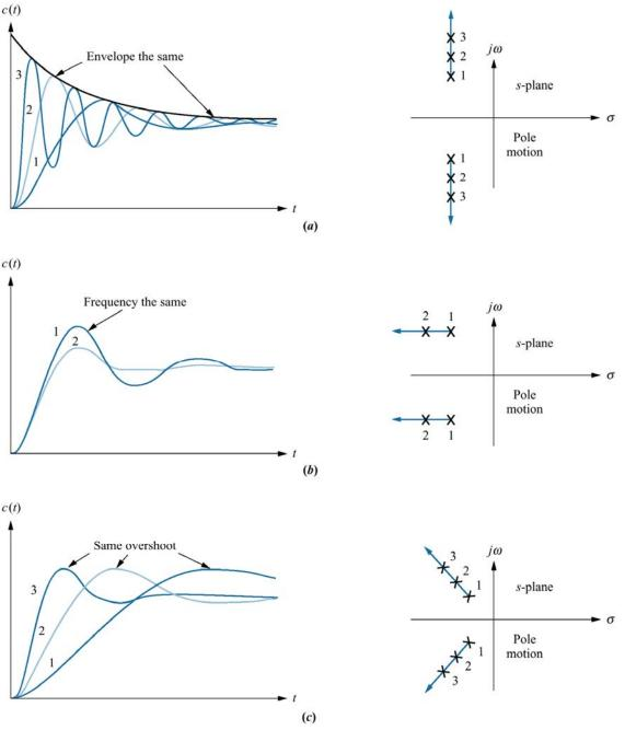
Step responses of second order underdamped systems as pole moves: (a) with constant real part, (b) with constant imaginary part, (c) with constant damping ratio.
