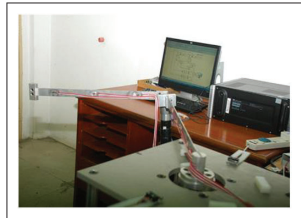
Figure 1. The experimental setup of a two-link flexible manipulator.
