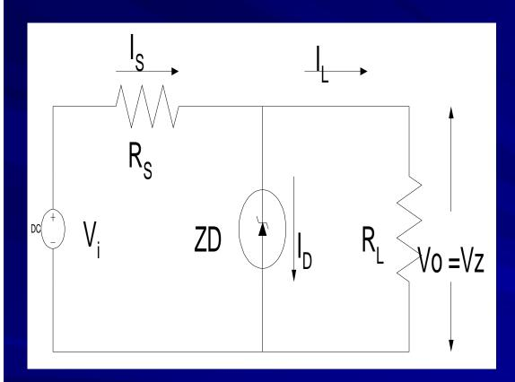
$$V_{i\min} = \frac{(R_L + R_S)V_Z}{R_L}$$
