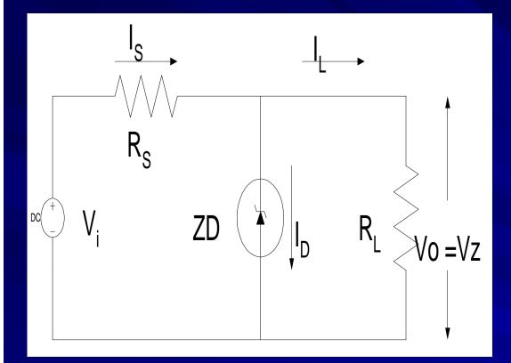
$$R_{L\min} = \frac{R_s V_z}{V_i - V_z}$$
