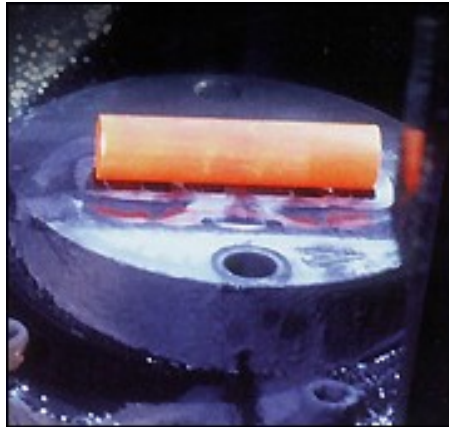
Gambar 2.1. Proses tempa ( www.muellerindustries.com )
