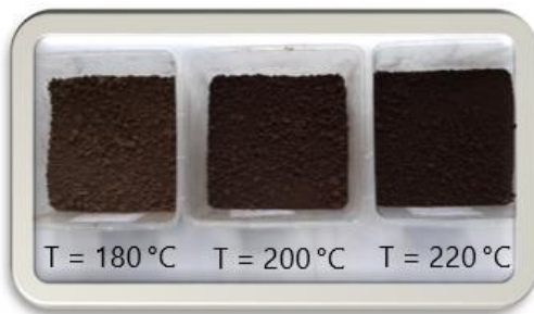
Fig. 6: Product appearance due to different final temperatures
