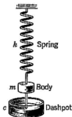
Fig. 35. Damped system
