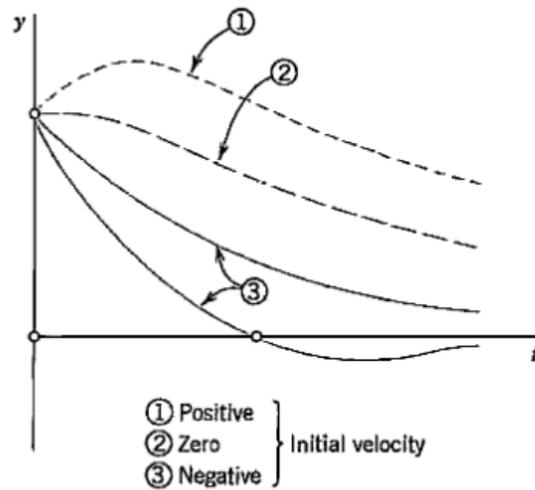
Fig. 37. Critical damping [see (8)]
