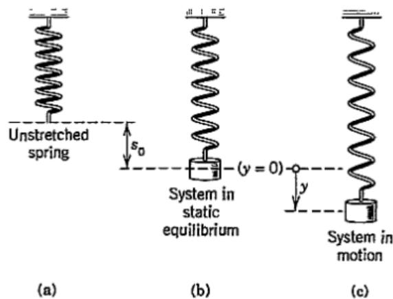
Fig. 32. Mechanical mass-spring system
