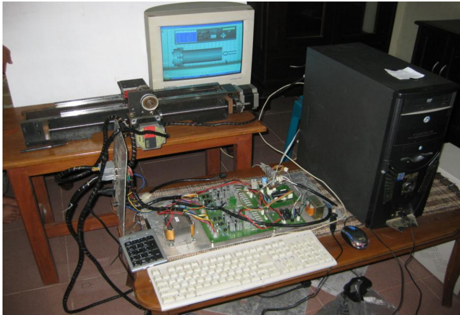
Gambar 4. Prototype Simulator CNC 2 Axis
